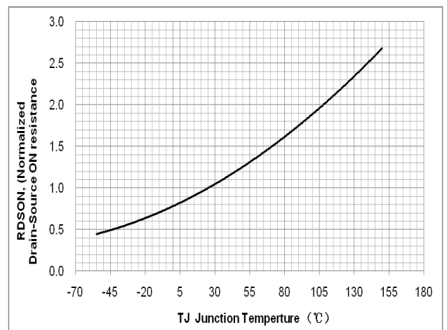
Fig. 6. On resistance variation vs. junction temperature
